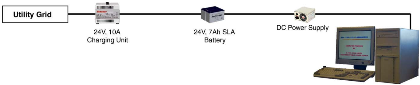
Fig. 2. Redesigned UPS without fuel cell system incorporated.
